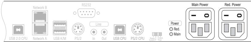
**Main Power:** Insert one of the supplied *PowerCable-2 Standard* IEC cables here.
