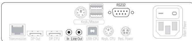
**NOTE:** By *default*, the KVM extender transfers audio data. The transmission of RS232 data is deactivated.
