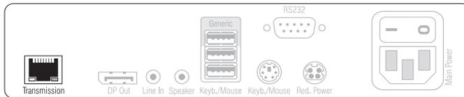
**Transmission:** Plug a category 5e (or better) twisted pair cable, which is available as accessory, into this interface. Connect the other end of the Gigabit Ethernet.
