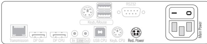
**Main Power:** Insert one of the supplied IEC cables here.
