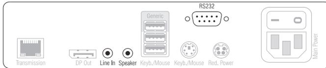
**Line In:** If required, connect a microphone to this interface.
