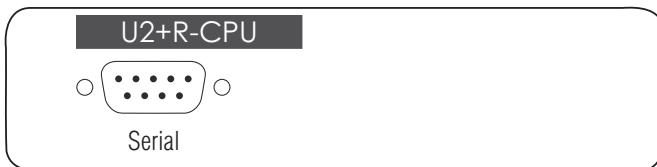
**Serial:** Use the RS232 cable to connect the computer's 9-pin serial computer interface to this interface (optional).
