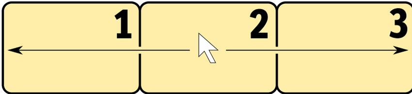
**EXAMPLE:** When moving the cursor to the right edge of **Monitor 2**, the KM switch switches to the module connected to **Monitor 3**.
