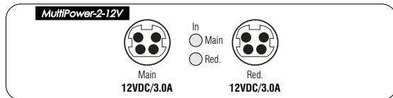
At least one external power supply (table power pack) supplies the voltage of the central power supply. A second, external power supply ensures uninterrupted operation if one of the two external power supplies fails.
