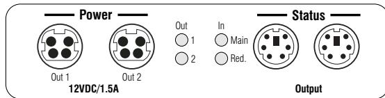
Use a power loop cable to connect the Mini-DIN 4 sockets of the two connectable devices to a Mini-DIN 4 socket of the central power supply.
