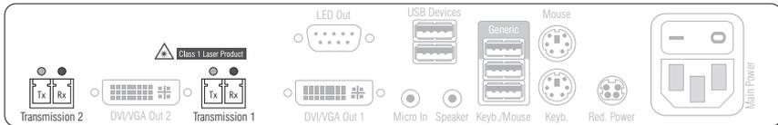
**Transmission 1 | Tx:** Insert the LC plug of a compatible optical fibre cable. Connect the other end of the cable to the **Rx** interface of a *Dynamic Port* provided at the matrix switch.
