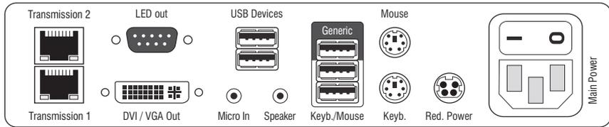
**DVI/VGA Out:** Connect the monitor/projector of the local console.
