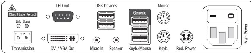
**NOTE:** Both keyboard and mouse signals can be transmitted to the computer using the PS/2 or the USB interfaces.
