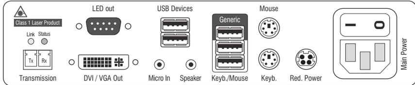
The back panel of the console module provides additional status LEDs. They have the following meaning:
