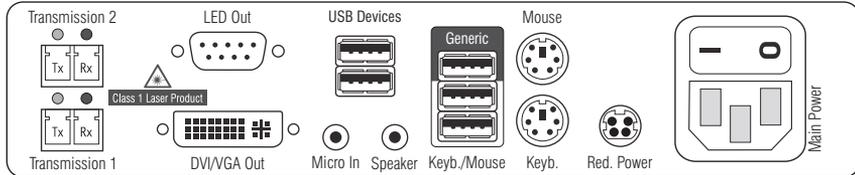
The *Transmission* interface at the back panel of the console module provides additional status LEDs. The LEDs have the following functions:
