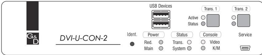
The LEDs on the front panel of the console module show the system's operating status.
