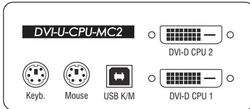
**NOTE:** Keyboard and mouse signals can be transmitted to the computer using *either* the PS/2 interfaces or the USB interface.
