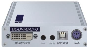
The data stream of the USB devices connected to the active console module (**DVI-U-CON** and **DP-U-CON** series only) is transmitted to the computer with up to 16 Mbit/s.
