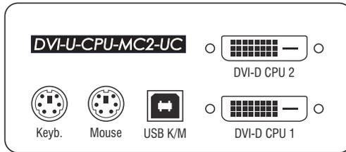
**NOTE:** Keyboard and mouse signals can be transmitted to the computer using *either* the PS/2 interfaces or the USB interface.
