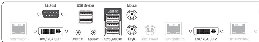
**DVI/VGA Out 1:** Connect the first console monitor.
