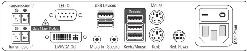
**DVI/VGA Out:** Connect the first console monitor.
