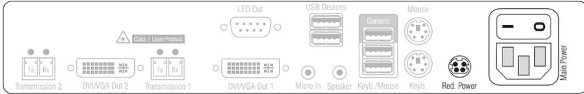
**Main Power:** Connect the supplied power cable. Insert the cable's Schuko plug in a power socket.
