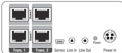
**Line In:** Use one of the supplied audio cables to connect the computer's *Line Out* interface to this interface.
