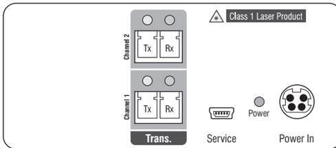
**Trans. | Channel 1 | Tx:** Insert the LC plug of a compatible optical fibre cable. Connect the other end of the cable to the **Rx** interface of a *Dynamic Port* provided at the matrix switch.
