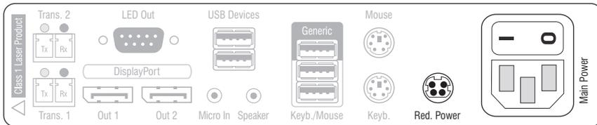
**Main Power:** Connect the supplied power cable. Insert the cable's Schuko plug in a power socket.
