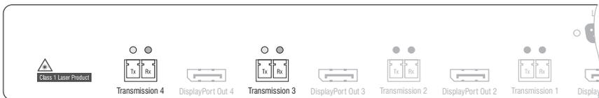
**Transmission 3 |Tx:** Insert the LC plug of a compatible optical fibre cable. Connect the other end of the cable to the **Rx** interface of a *Dynamic Port* provided at the matrix switch.
