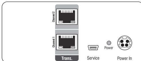
**Trans. | Channel 1:** Connect this interface to a *Dynamic Port* (RJ45) of the matrix switch.
