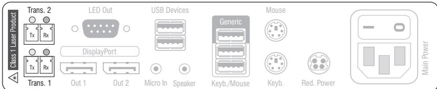
**Transmission 1 | Tx:** Insert the LC plug of a compatible optical fibre cable. Connect the other end of the cable to the **Rx** interface of a *Dynamic Port* provided at the matrix switch.
