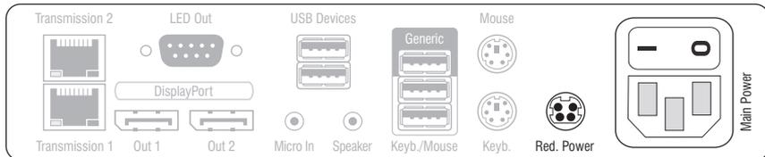
**Main Power:** Connect the power cable to the power pack and a power outlet.
