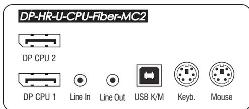
**DP CPU 1:** Use one of the supplied video cables to connect the computer's first *Display Port* video output to this interface.
