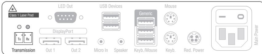
**Transmission | Tx:** Insert the LC plug of a compatible optical fibre cable. Connect the other end of the cable to the **Rx** interface of a *Dynamic Port* provided at the matrix switch.
