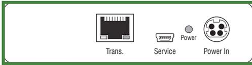
**Trans.:** Connect this interface to a *Dynamic Port* (RJ45) of the matrix switch.
