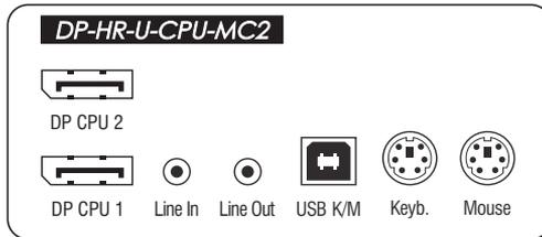
**DP CPU 1:** Use one of the supplied video cables to connect the computer's first *Display Port* video output to this interface.
