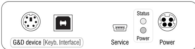
**G&D device:** Use the supplied PS/2 or USB connection cable to connect this interface and the PS/2 or USB keyboard interface of the compatible G&D device.
