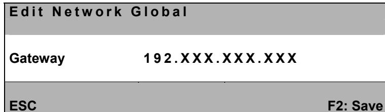
Now enter the IP address of the gateway on the gateway row. To do so, use either the **right arrow / left arrow** keys or the **TAB** key to move to one of the four fields. Press the **ENTER** key to activate edit mode in each individual field; the font color changes to yellow.
