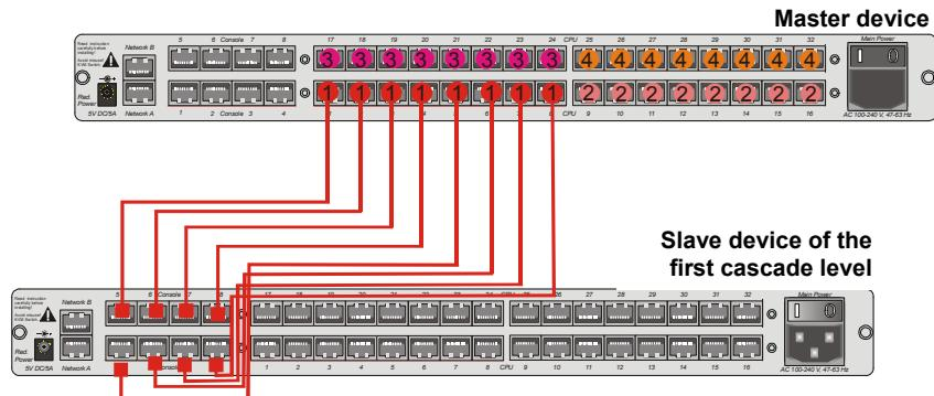
The CPU ports 1 – 8 are connected to the slave device with one CAT cable each (that is, with a total of 8 CAT cables). These CAT cables are attached to the RJ45 console connection ports on the slave device.
