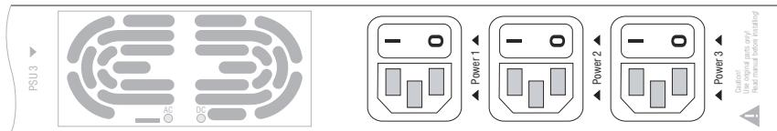
**Power x:** Connect one of the supplied power cables for each installed power supply module. Connect the power cable with a power socket and turn on the power switch.
